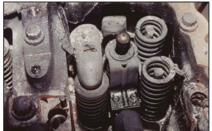
Photo 8 - Damaged Valve Components (South Engine)
