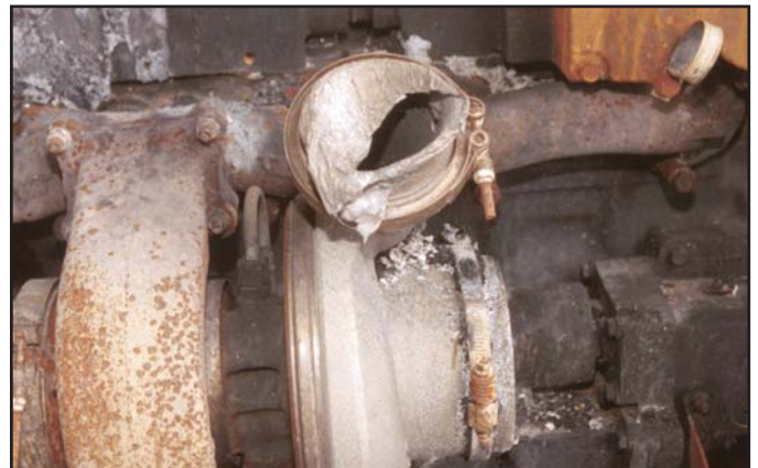
Photo 12 - Fire Damaged Turbocharger Outlet Elbow (North Engine)
