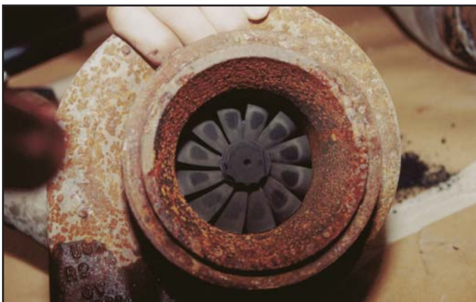
Photo 4a - Turbocharger Impeller (South Engine) Scrubbed Clean
