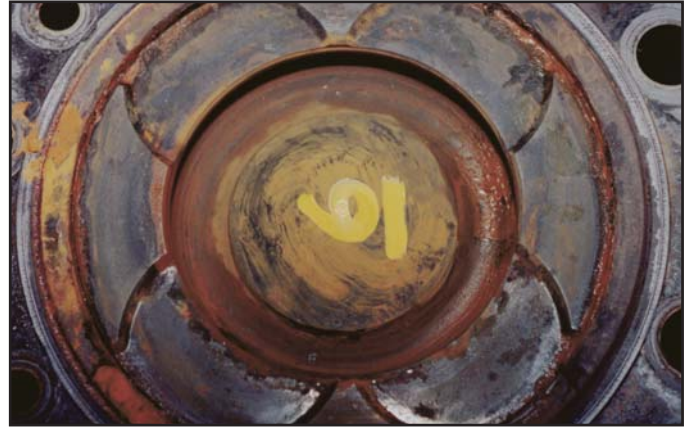
Photo 6 - Piston Valve Contact (South Engine)
