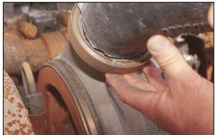
Photo 11b - Turbocharger Outlet Elbow (South Engine) Mechanical Failure
