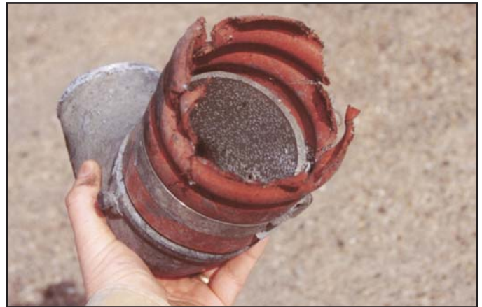
Photo 11a - Turbocharger Outlet Rubber Hose Connection (South Engine) Mechanical Failure
