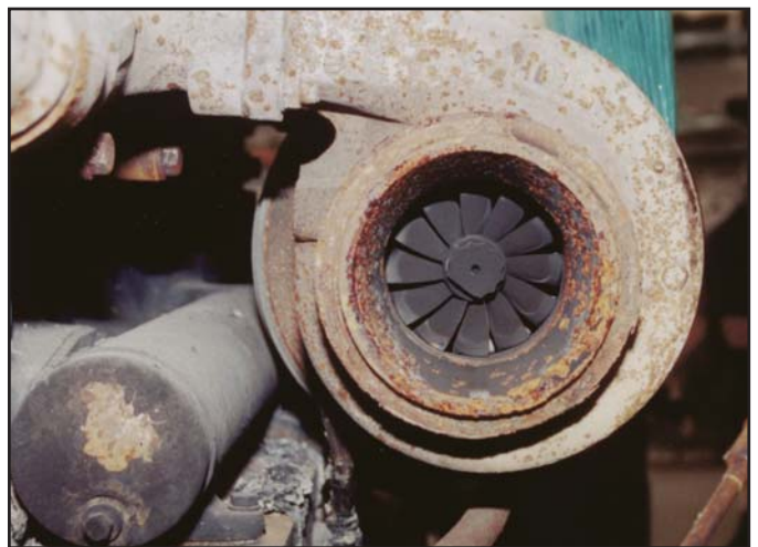
Photo 2 - Turbocharger Impeller (North Engine) Soot Covered
