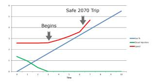
This standard engine configuration, with turbocharger, was operated at 7% load. The fuel rate is therefore low and drops to zero quickly. Runaway begins at a gas level of just 1.4% (28% of LEL), and the engine accelerates beyond the red line only 5.5 seconds later. The automatic system operates when the gas is at 3.6% (72% of LEL). In this situation there is little time for manual operation of any intake shutdown device, and only automatic sensing will prevent an explosion.
